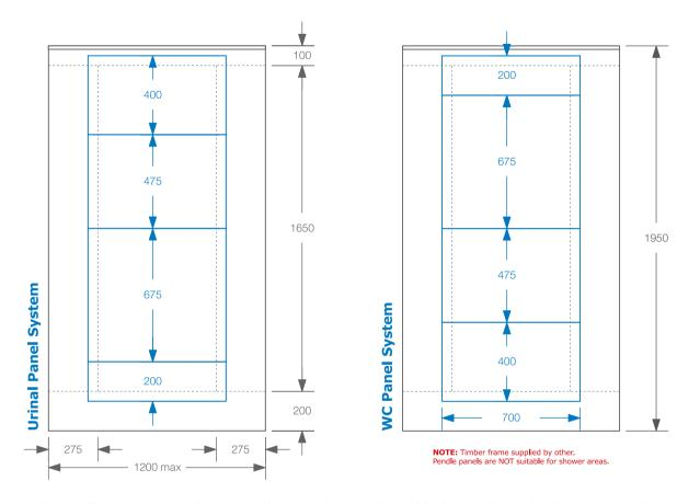
The Pendle washroom panel system has been developed for both Urinal and WC panel configurations. With an overall height to match a Pendle Toilet Cubicle, this box packed panel system can be cut-to-size on site to fit various cubicle widths up to a max of 1200mm.
